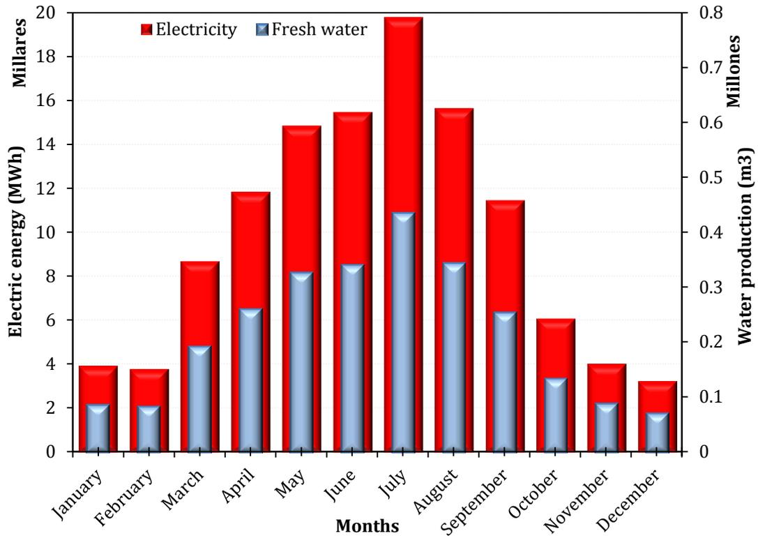
Figure 27: Monthly electrical net power and fresh water generated from the proposed plant.
