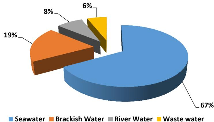
**Figure 2: Worldwide feed-water percentage used in desalination [5].**
