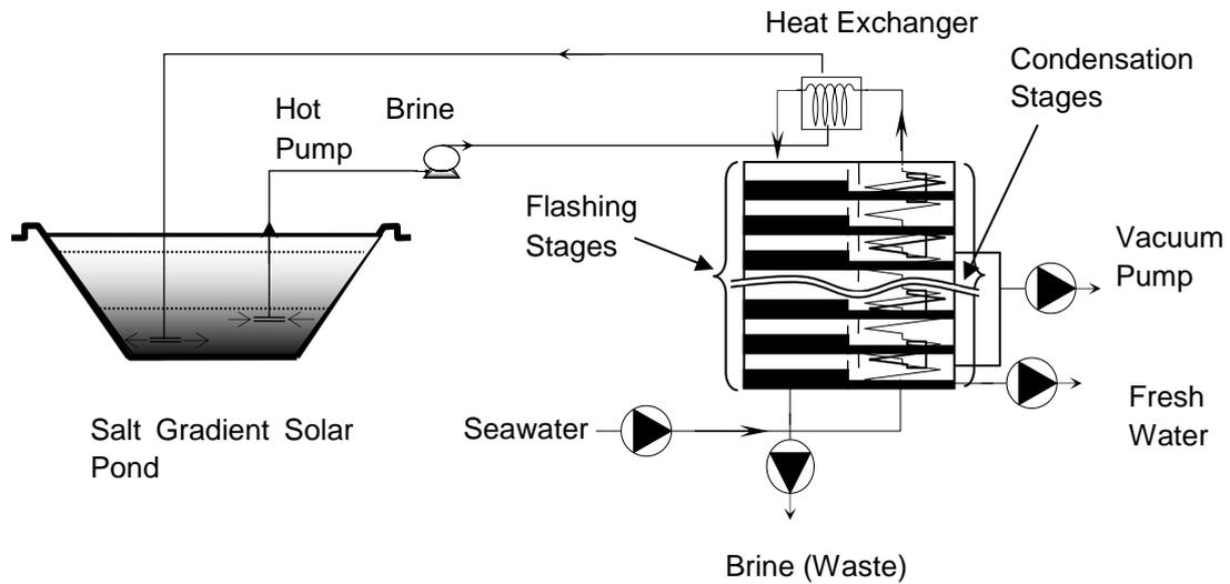
**Figure 14: Schematic drawing of MSF Desalination Unit coupled with the Tajoura Experimental Solar Pond (TESP).**
